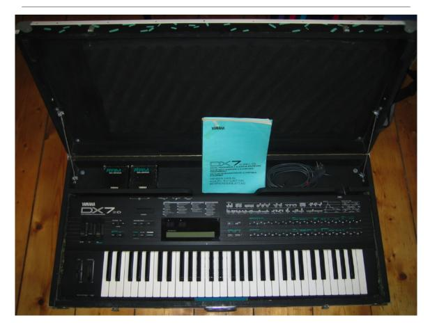
**Figure 4.1:** Yamaha DX7 synthesizer, the first commercially successful instrument to offer FM synthesis, digital synthesis, and MIDI compatibility. The instrument pictured here is packaged in a road case. Photographer: schoschie (http://www.flickr.com/photos/schoschie/51653026/<sup>5</sup>). Copyright holder has granted permission to display this image under the Creative Commons Attribution-ShareAlike license<sup>6</sup>.
