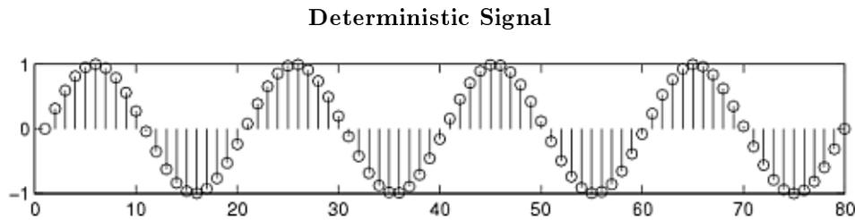
**Figure 1:** An example of a deterministic signal, the sine wave.
