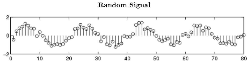
**Figure 2:** We have taken the above sine wave and added random noise to it to come up with a noisy, or random, signal. These are the types of signals that we wish to learn how to deal with so that we can recover the original sine wave.
