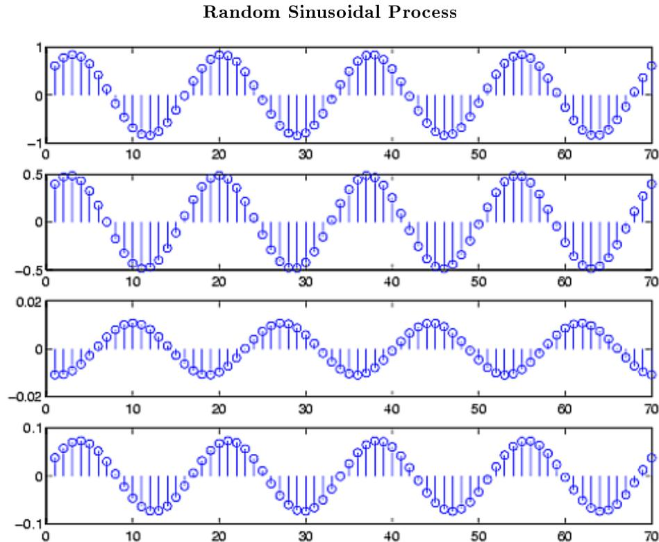
**Figure 3:** A random sinusoidal process, with the amplitude and phase being random numbers.
