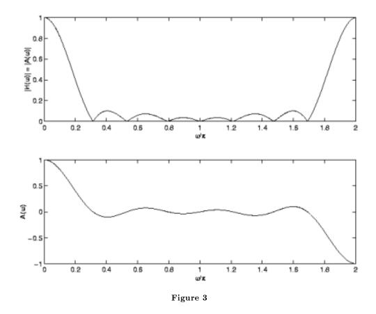
The following Matlab code fragment produces a plot of  $A(\omega)$  for a Type II FIR filter.
