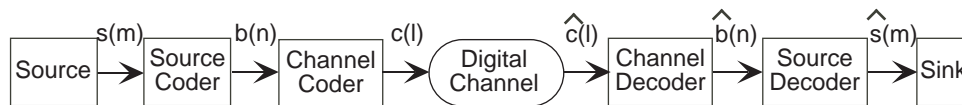
Figure 1: To correct errors that occur in the digital channel, a channel coder and decoder are added to the communication system. Properly designed channel coding can greatly reduce the probability (from the uncoded value of p_e ) that a data bit b(n) is received incorrectly even when the probability of c(l) be received in error remains p_e or becomes larger. This system forms the Fundamental Model of Digital Communication.
