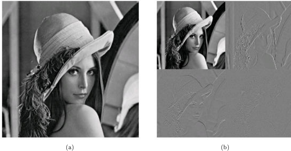
Figure 1: Original Figure 1(a) and the Level 1 Haar transform Figure 1(b) of the 'Lenna' image.
