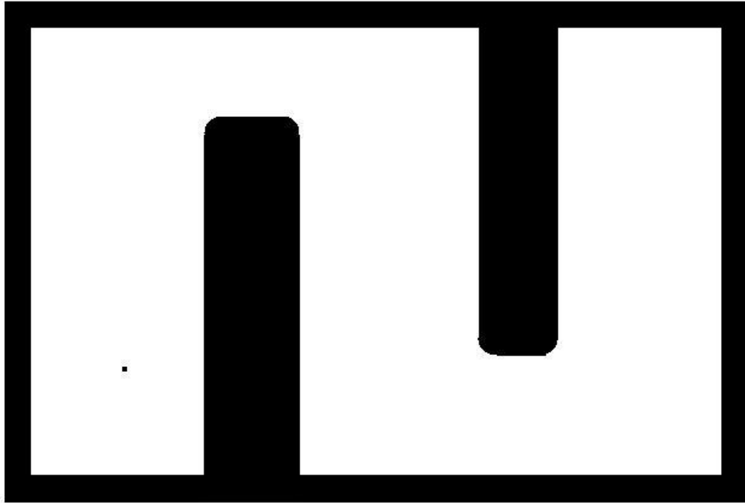
Figure 3: The configuration space corresponding to the above work space. Each point now corresponds to a configuration of the robot, rather than a real point in space. To see how it was constructed, choose any point on the robot as a reference. Now imagine the curves swept out by that point as the robot slides along the surface of the obstacles and along the border of the work space. Every configuration closer to the obstacles than this curve is in collision, and every configuration farther than the curve is free.
