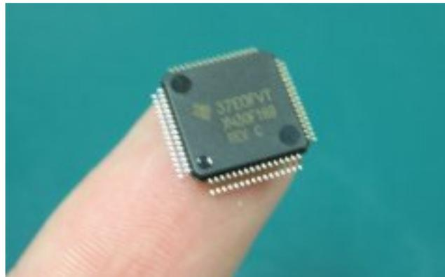
**Figure 1:** The TI MSP430F169 meets the criteria we listed above and is a good example of a modern microcontroller.
