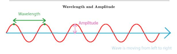
Figure 1: The wavelength is the distance between the "crests" of two waves that are next to each other. The amplitude is how high the crests are.
