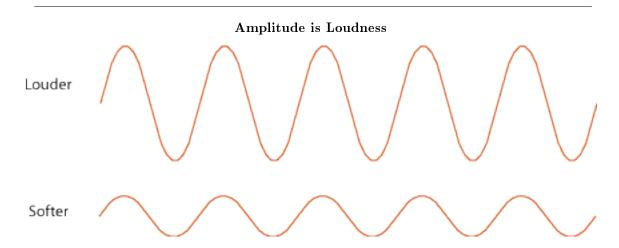
Figure 3: The size of a wave (how much it is "piled up" at the high points) is its amplitude. For sound waves, the bigger the amplitude, the louder the sound.
