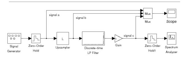
Figure 6: Simulink model for discrete-time interpolation.
