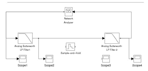
Figure 5: Initial Simulink model for sampling and reconstruction using a sample-and-hold. This system only measures the frequency response of the analog filters.
