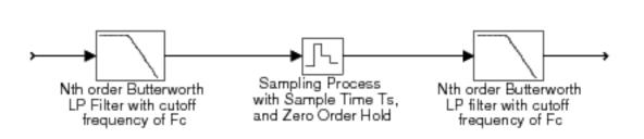
Figure 2: Sampling and reconstruction using a sample-and-hold.
