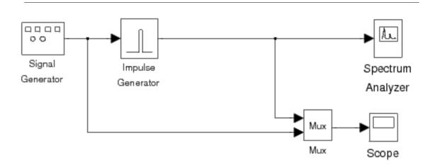
Figure 4: Simulink model for sampling and reconstruction using an impulse generator.
