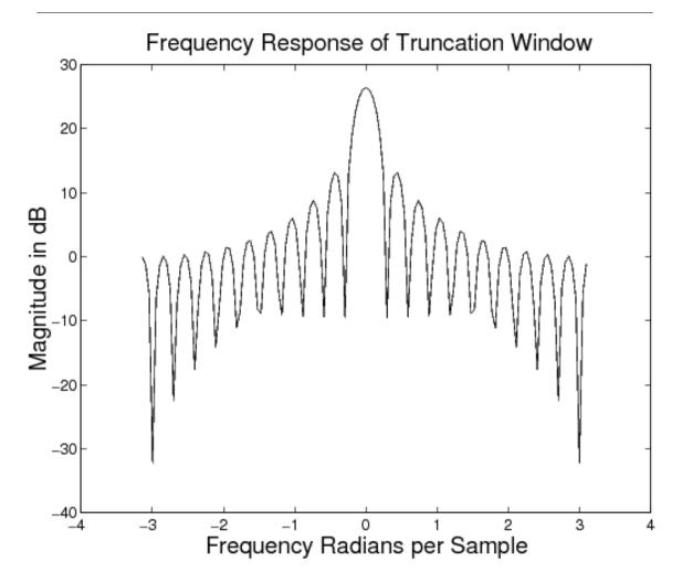
Figure 7: DTFT of a rectangular window of size 21.
