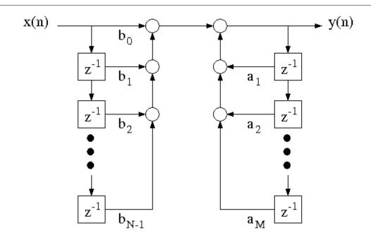
Figure 1: Direct form implementation for a discrete-time filter described by a linear recursive difference equation.
