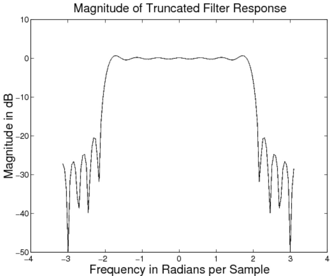
**Figure 2:** Frequency response of low-pass filter, designed using the truncation method.
