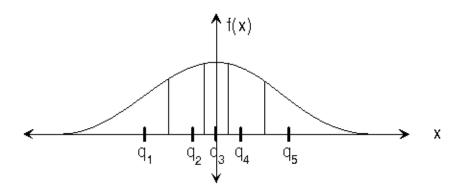
Figure 2: Five level Max quantizer for Gaussian-distributed signal.
