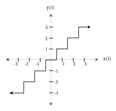
Figure 1: Input-output relation for a 7-level uniform quantizer.
