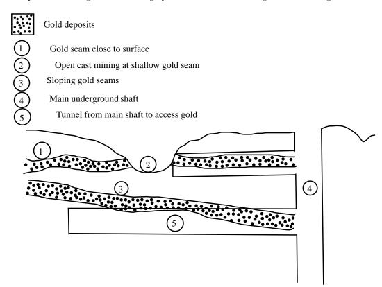
Figure 2: Diagram showing open cast and shaft mining
