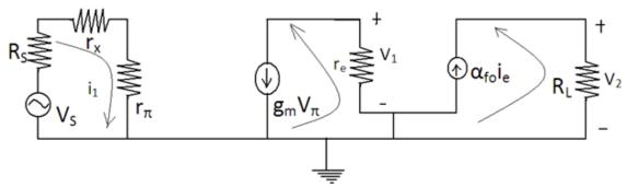
Figure 4. Midfrequency incremental model of CASCODE AMPLIFIER.
