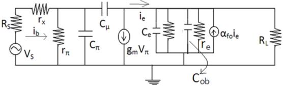
Figure 3. The incremental model of Cascode Amplifier with CE BJT being replaced by Hybrid-pi Model and CB BJT being replaced by T-Model. This is high frequency Model.
