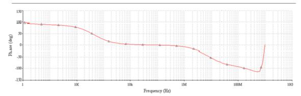
Figure 3.b. Phase of Gain vs frequency plot of CB Amplifier. y-axis: Phase of Gain in degrees; x-axis: frequency plot on logrithmic scale.
