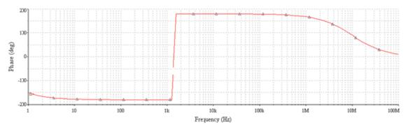
Figure 2b. Phase of the Gain of Emitter Degenerate Amplifier vs Frequency Response Curve. y-axis:Phase of Gain in degrees; x-axis: logrithmic plot of frequency in Hz;
