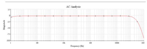
Figure 4. Gain Magnitude Plot in dB of CC Amplifier. y-axis: Gain Magnitude in dB; x-axis: Frequency plot on logrithmic scale.
