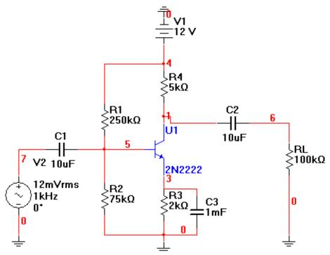
Figure 1.c. Circuit Schematics of CE Amplifier.
