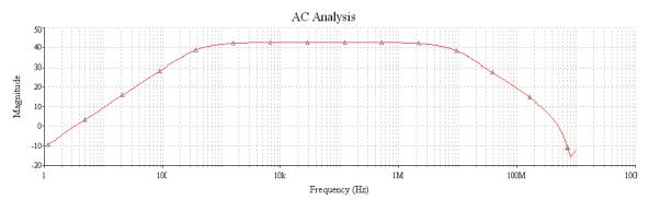
Figure 3. Gain Magnitude Frequency Response Curve of CB Amplifier y-axise: Gain Magnitude in dB; x-axis: Frequency Plot on logrithmic scale;
