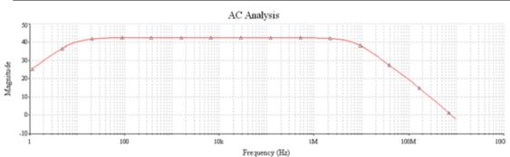
Figure 1. Gain Magnitude Frequency Response Curve of CE Amplifier. y-axis: Gain Magnitude in dB;
