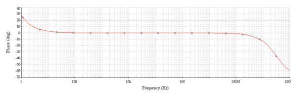
Figure 4.b. Phase of Gain of CC Amplifier vs Frequency. y-axis: Phase of Gain in degrees; x-axis: Frequency Plot on logrithmic scale.
