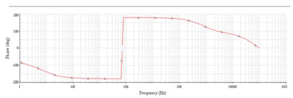
Figure 1.b. Phase of Gain vs Frequency of CE Amplifier.
