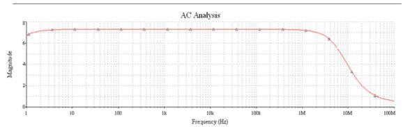
Figure 2. Gain Magnitude Frequency Response Curve of Emitter Degenerate Amplifier. y-axis: Gain Magnitude in dB; x-axis: logrithmic frequency plot in Hz;
