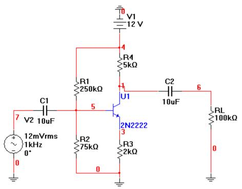
Figure 2.c.Circuit Schematics of Emitter Degenerate Ampl.
