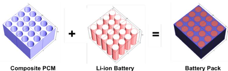
**Figure 7: Application with PCM Technology.** A pack of Li-ion batteries kept at a narrow temperature range with a proper use of passive thermal management system. *Source: AllCell's PCM Technology©*
