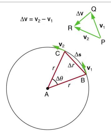
Figure 1: The directions of the velocity of an object at two different points are shown, and the change in velocity  $\Delta v$  is seen to point directly toward the center of curvature. (See small inset.) Because  $a_c = \Delta v/\Delta t$ , the acceleration is also toward the center;  $a_c$  is called centripetal acceleration. (Because  $\Delta \theta$  is very small, the arc length  $\Delta s$  is equal to the chord length  $\Delta r$  for small time differences.)
