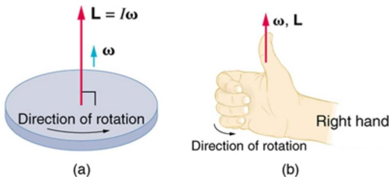
**Figure 1:** Figure (a) shows a disk is rotating counterclockwise when viewed from above. Figure (b) shows the right-hand rule. The direction of angular velocity  $\omega$  size and angular momentum  $L$  are defined to be the direction in which the thumb of your right hand points when you curl your fingers in the direction of the disk's rotation as shown.
