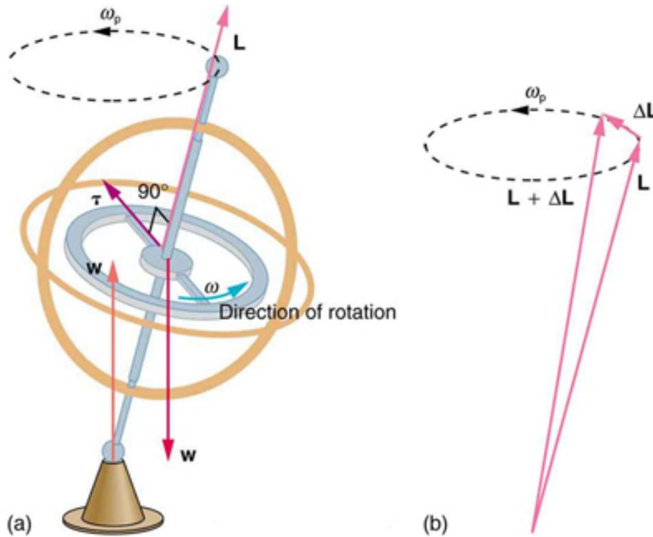
**Figure 4:** As seen in figure (a), the forces on a spinning gyroscope are its weight and the supporting force from the stand. These forces create a horizontal torque on the gyroscope, which create a change in angular momentum  $\Delta L$  that is also horizontal. In figure (b),  $\Delta L$  and  $L$  add to produce a new angular momentum with the same magnitude, but different direction, so that the gyroscope precesses in the direction shown instead of falling over.
