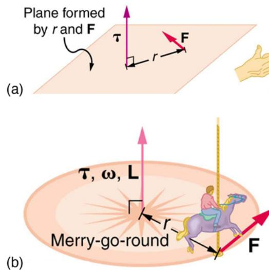
**Figure 2:** In figure (a), the torque is perpendicular to the plane formed by  $r$  and  $F$  and is the direction your right thumb would point to if you curled your fingers in the direction of  $F$ . Figure (b) shows that the direction of the torque is the same as that of the angular momentum it produces.
