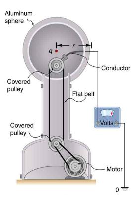
Figure 1: The voltage of this demonstration Van de Graaff generator is measured between the charged sphere and ground. Earth's potential is taken to be zero as a reference. The potential of the charged conducting sphere is the same as that of an equal point charge at its center.
