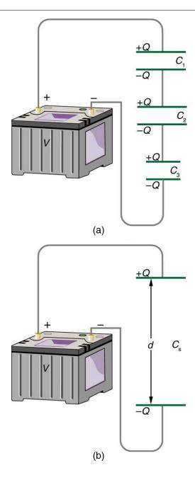
**Figure 1:** (a) Capacitors connected in series. The magnitude of the charge on each plate is Q. (b) An equivalent capacitor has a larger plate separation d. Series connections produce a total capacitance that is less than that of any of the individual capacitors.
