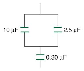
Figure 4: A combination of series and parallel connections of capacitors.
