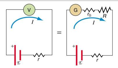
Figure 1: An analog voltmeter attached to a battery draws a small but nonzero current and measures a terminal voltage that differs from the emf of the battery. (Note that the script capital E symbolizes electromotive force, or emf.) Since the internal resistance of the battery is not known precisely, it is not possible to calculate the emf precisely.
