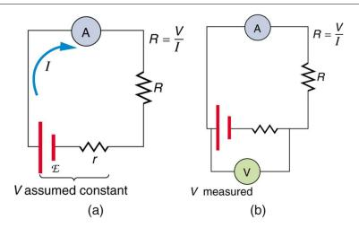
**Figure 3:** Two methods for measuring resistance with standard meters. (a) Assuming a known voltage for the source, an ammeter measures current, and resistance is calculated as  $R = \frac{V}{I}$ . (b) Since the terminal voltage V varies with current, it is better to measure it. V is most accurately known when I is small, but I itself is most accurately known when it is large.
