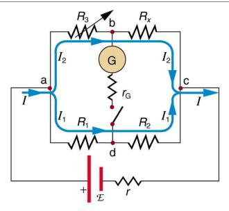
Figure 4: The Wheatstone bridge is used to calculate unknown resistances. The variable resistance  $R_3$  is adjusted until the galvanometer reads zero with the switch closed. This simplifies the circuit, allowing  $R_x$  to be calculated based on the IR drops as discussed in the text.
