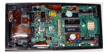
Figure 1: Energy stored in the large capacitor is used to preserve the memory of an electronic calculator when its batteries are charged. (credit: Kucharek, Wikimedia Commons)
