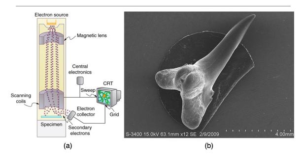
Figure 2: Schematic of a scanning electron microscope (SEM) (a) used to observe small details, such as those seen in this image of a tooth of a *Himipristis*, a type of shark (b). (credit: Dallas Krentzel, Flickr)
