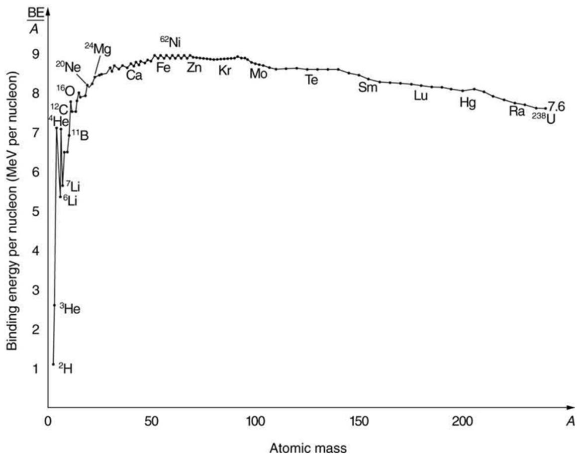
**Figure 3:** A graph of average binding energy per nucleon,  $BE/A$ , for stable nuclei. The most tightly bound nuclei are those with  $A$  near 60, where the attractive nuclear force has its greatest effect. At higher  $A$ s, the Coulomb repulsion progressively reduces the binding energy per nucleon, because the nuclear force is short ranged. The spikes on the curve are very tightly bound nuclides and indicate shell closures.
