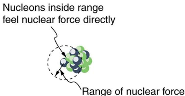
**Figure 4:** The nuclear force is attractive and stronger than the Coulomb force, but it is short ranged. In low-mass nuclei, each nucleon feels the nuclear attraction of all others. In larger nuclei, the range of the nuclear force, shown for a single nucleon, is smaller than the size of the nucleus, but the Coulomb repulsion from all protons reaches all others. If the nucleus is large enough, the Coulomb repulsion can add to overcome the nuclear attraction.
