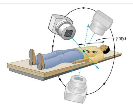
Figure 2: The  $^{60}$ Co source of  $\gamma$ -radiation is rotated around the patient so that the common crossing point is in the tumor, concentrating the dose there. This geometric technique works for well-defined tumors.
