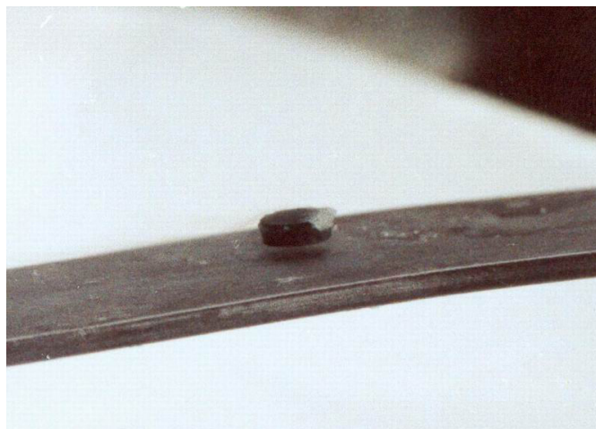
Figure 2: One characteristic of a superconductor is that it excludes magnetic flux and, thus, repels other magnets. The small magnet levitated above a high-temperature superconductor, which is cooled by liquid nitrogen, gives evidence that the material is superconducting. When the material warms and becomes conducting, magnetic flux can penetrate it, and the magnet will rest upon it. (credit: Saperaud)
